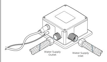
Please wait approximately 60 seconds after connecting the sensor cable for sensor calibration to complete and to begin using the faucet.
